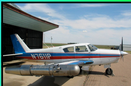
Wingtip Generator for Rain Increase & Hail Suppression / 42 Grams
